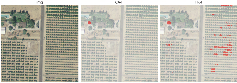
FIG. 10. Example of false predictions of PV by the FR-I trained model on the rows of agricultural activity seen in CA-F.
