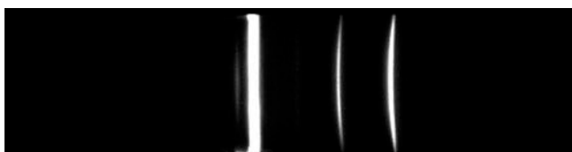
Figure 6 Sample spectrum taken of dry room air, showing the spatial effects of coma and vignetting. The three major features visible in the spectrum are from left-to-right: (1) rotational N_2 and O_2 scattering adjacent to the laser line, (2) vibrational O_2 , (3) vibrational N_2 .
