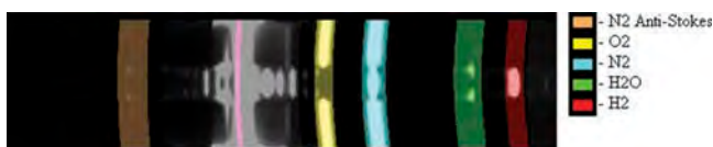
Figure 7 Sample spectrum of the dilute diffusion flame with spatial corrections and background subtraction applied. Spectrum is an average of 100 shots taken at 5.5 mm axially from the nozzle. Horizontal dimension is wavelength and vertical dimension is spatial distance along the laser probe length. Color overlays show the calculated bin locations for each specie. Fuel is indicated along the centerline with air bounding it on the top and bottom. Water (indicating reaction) is present in the interface.
